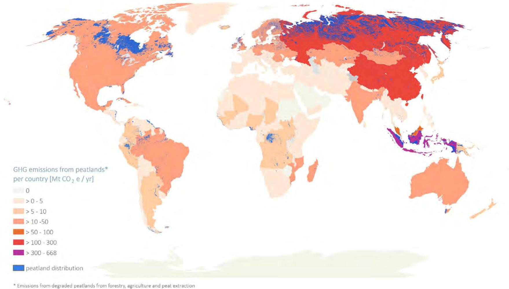
Figure 2.10. Emissions from peatlands degraded by forestry, agriculture and peat extraction per country (microbial respiration only, without fire; including CO<sub>2</sub>, CH<sub>4</sub>, N<sub>2</sub>O, DOC, and emissions from ditches. Data have been derived from multiple sources. Numbers may change with future assessments, but the order of magnitude will probably stay the same for many countries (especially for developed countries and main emitters).
