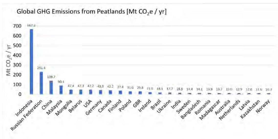
Figure 0.3: Estimated global greenhouse gas emissions from degraded peatlands from top 25 countries. Calculations are based on the peatland drained area for forestry, agriculture and peat extraction and IPCC (2014) emission factors including CO<sub>2</sub>, CH<sub>4</sub>, N<sub>2</sub>O, DOC, and emissions from ditches. Includes only net, on-site GHG emissions. Wildfire emissions are not included.
