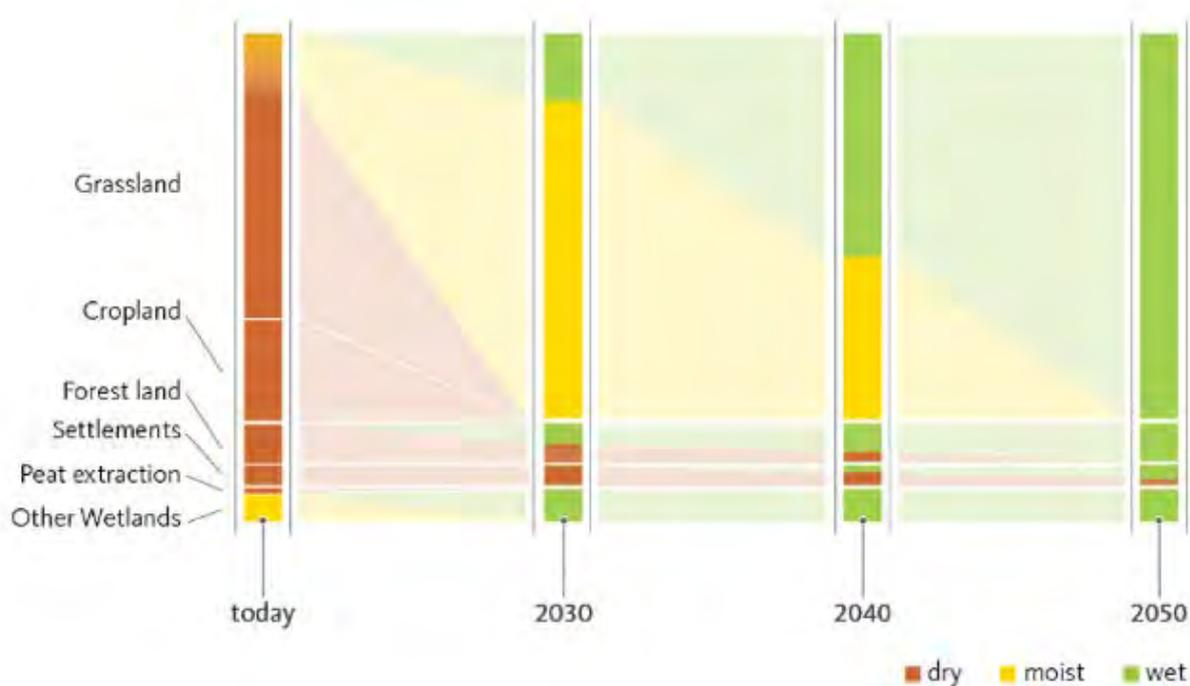
Figure 5.13. Net zero CO<sub>2</sub> emission pathway for organic soils in Germany visualising transformation by land use category (in % of total area of organic soils) over the period 2020–2050 (pathway 1). Dry=deep-drained, moist=shallow-drained (mean annual water table ~ 30 centimetres below soil surface), wet=undrained/rewetted (mean annual water table at the soil surface).
