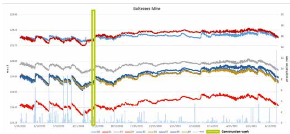
Figure 56 . Water level fluctuations in Baltezers peatland before and after the building of dams. In 2020, improvements were made to the measurement system with additional equipment that displays more accurate and reliable data, therefore only this period is presented here.
