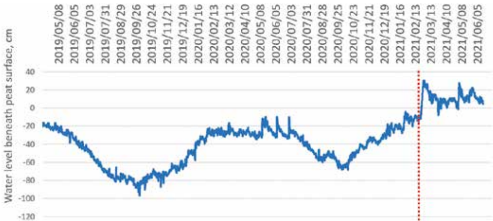
Figure 131. Water level dynamics in Amalva peatland, in 2019–2021. Red line indicates the time of dam construction, i.e. finishing the rewetting actions.
