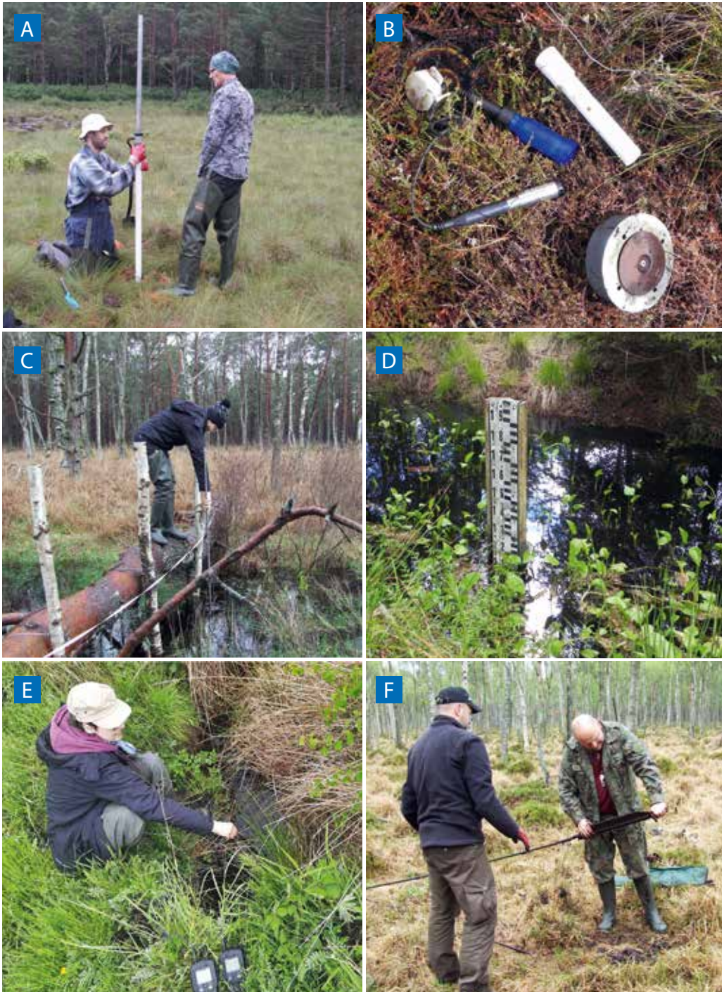
Figure 92. Field work: A – installation of piezometers; B – reading data from divers; C – water flow measurement; D – reading the water level from the gauge; E – in situ measurements of surface water parameters; F – collection of peat cores. Photos: I. Chlost (A, B, D, F); M. Pawłowska (E), I. Bubak (C).
