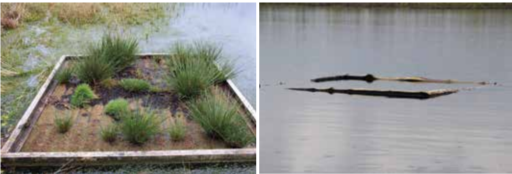
Figure 99. Other prototypes after testing time. On the left – the island which lost anchoring and drifted to the shore (one year since launching in May 2020); on the right – the island which lost buoyancy after two years, May 2020. Photos: K. Bociąg.
