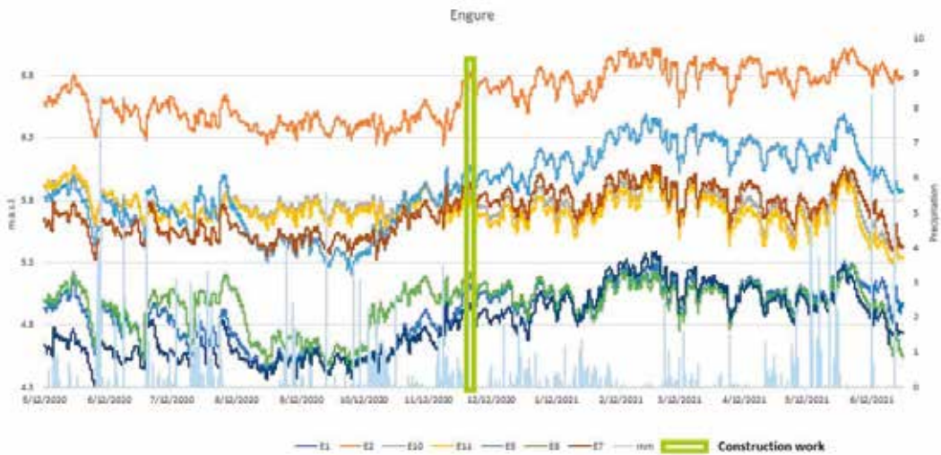
Figure 48. Water level fluctuations in the Engure restoration area (the water level is presented above the sea level), from December 2020 to June 2021. In 2020, improvements were made to the measurement system with additional equipment that displays more accurate and reliable data, therefore only this period is presented here.
