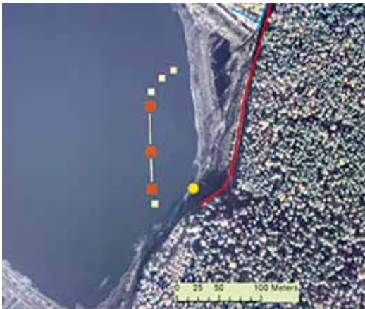
Figure 109. Arrangement of the floating islands on the eastern part of the post-excavating water basin. Red square (on the left picture) – a set of 12 islands (No. 1 in the figure to the right); white square – a set of 8 islands (2), lines – sets of 13 (3) and 10 (4) islands.
